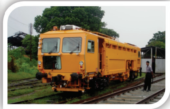
Tamping machine before using for maintenance work.
