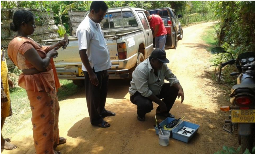
Measuring EC as in-situ test in the field areas.
