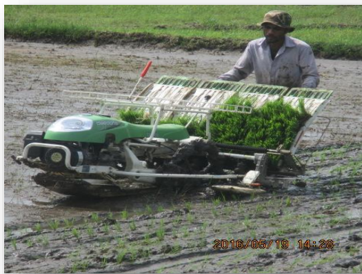
Mechanized transplanting of paddy Injinimitiya Scheme
