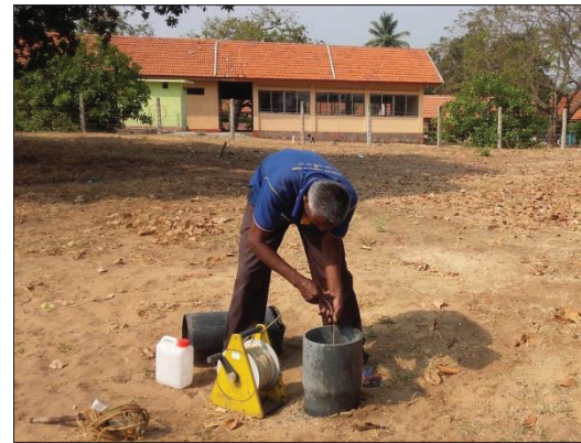
Figure 02: Water level monitoring and water sample collection
