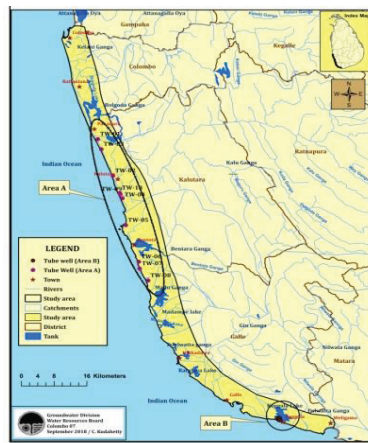
Figure 03 - 1: Established groundwater monitoring network areas, sampling and water level monitoring points (Colombo to Weligama coastal strip)
