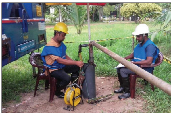
Figure 5 & 6: Conducting a pumping test at Mathale
