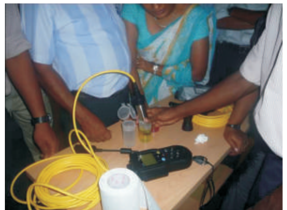
Field measurement of NO 3 in groundwater
