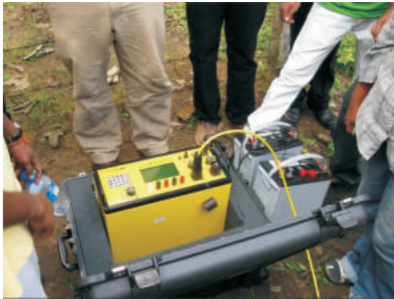
AGI equipment set up for geophysical survey
