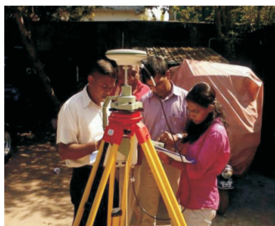
Establishment of base station
