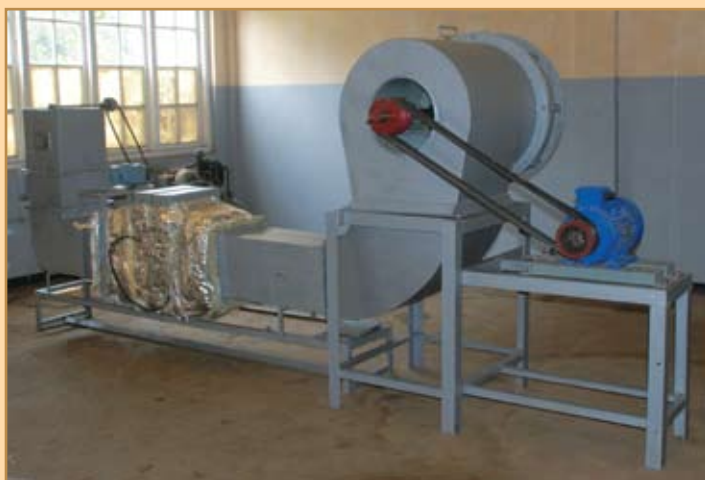
Pilot scale experimental Fluidized Bed Drier (FBD) unit
