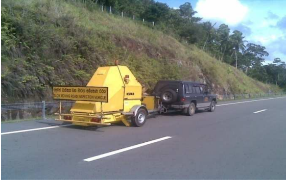
FWD Surveying on STDP
