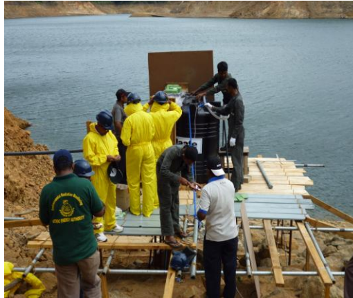
Fig No. 03: Set up for release of I-131 radioactive tracer to the Samanalawewa resourvior
