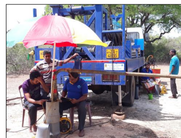
Fig 19: Conducting pumping test for a tube well of CBO
