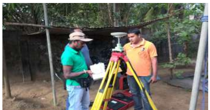
Fig7: In-situ chemical testing of groundwater and well leveling for assessment groundwater flow pattern of the area
