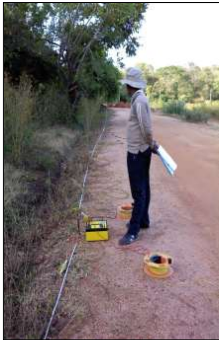
Conducting 1D Resistivity surveys
