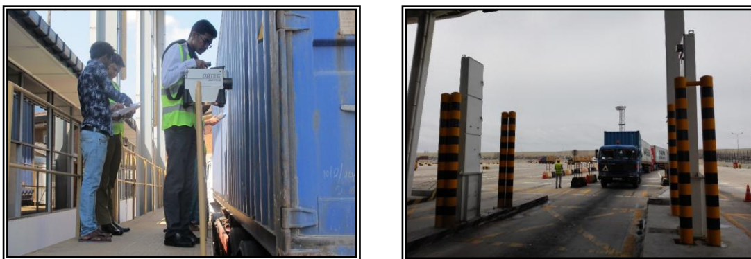
Figure 5: Radiation monitoring of shipping containers at the Colombo port
