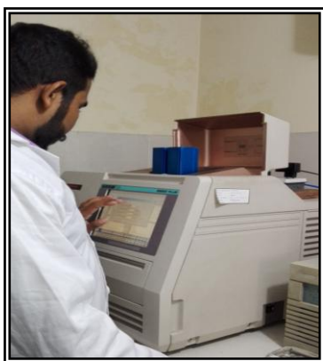
Figure: 1 Reading a Dosimeter using TLD Reader
