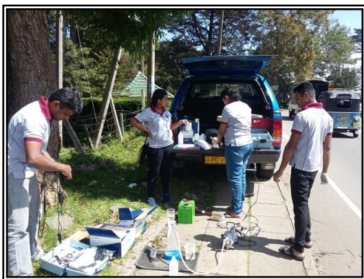
Figure 8: Filtration of water samples collected for Nitrogen Isotope Analysis
