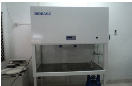
Lamina-flow cabinet for microbiology experiments
