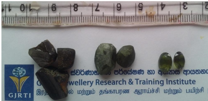
Figure 6. Image is showing left- unheated low value zircon samples, middle- heated samples in reducing atmospheric condition and right- heated cut and polished samples.
