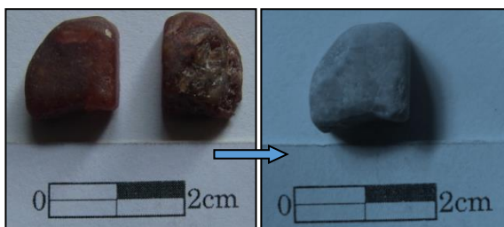
Figure7. Reddish brown zircon became blue when treated at 1100 0 C in reducing atmosphere
