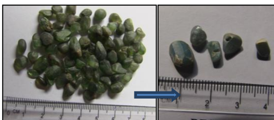
Figure 8. Greenish zircon became pale blue when treated at 1750 0 C in reducing atmosphere
