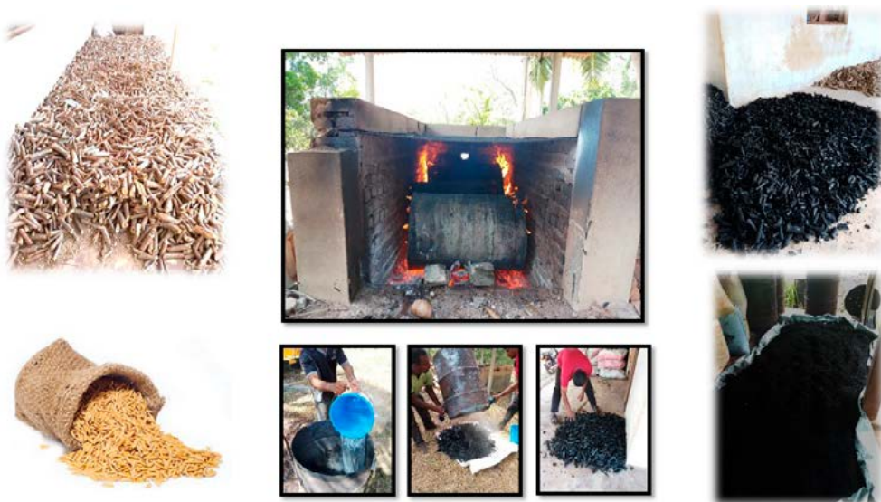
Production of Gliricidia stick and paddy husk biochar using Artisanal Biochar production technique
