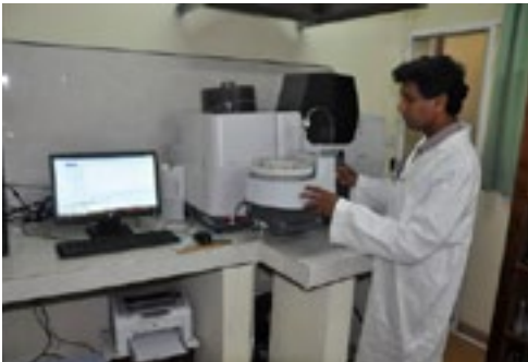
Leaf sample analysis for DFR using Atomic Absorption Spectrophotometer
