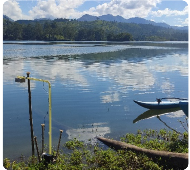
Onsite Wave Height Monitoring (Sensor Based)
