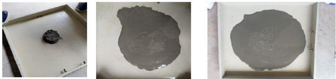
a) Water/Cement: 0.4 + 1% coir b) Water/Cement: 0.6 + 1% coir c) Water / Cement: 0.7 + 1% coir
