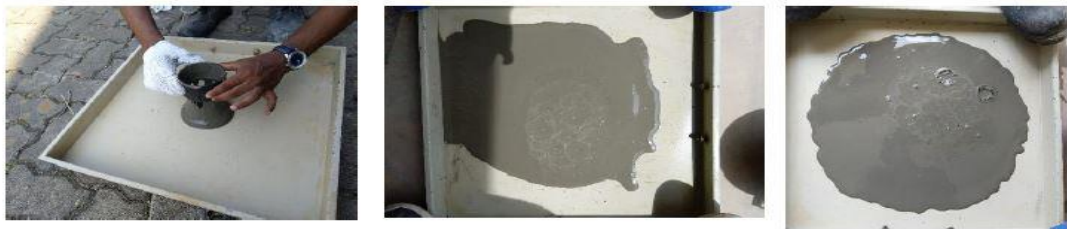
a) Water/Cement: 0.4 b) Water/Cement: 0.6 c) Water / Cement: 0.7 Figure 4: Flowability with increased water cement ratio of a plain mixture
