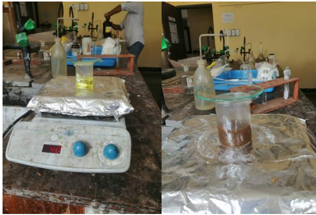
Figure 12 – Carrying out experiments to produce a coloured gold alloy
