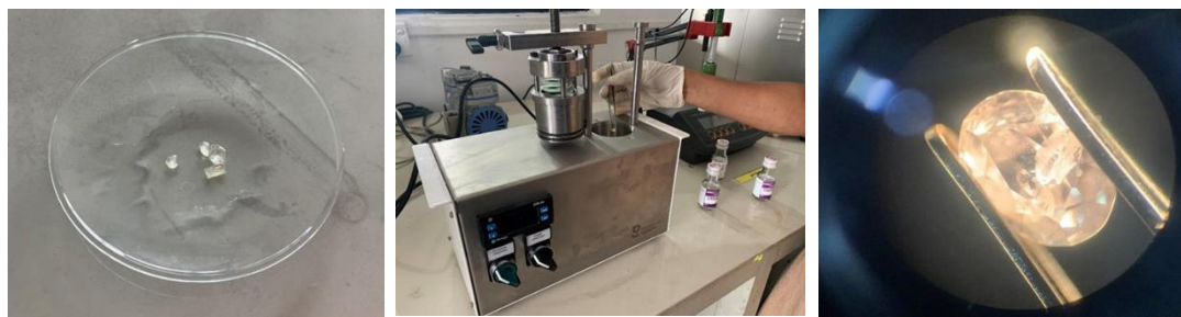
Figure 11 - Conducting research to identify a suitable oil for filling cracks
