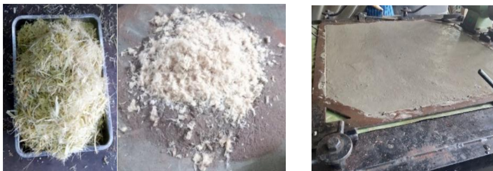
Visual observation of shaded cornhusk and pre-treated fibres from AHP Composite mixture spread on iron mould in a bed of a vibration machine
