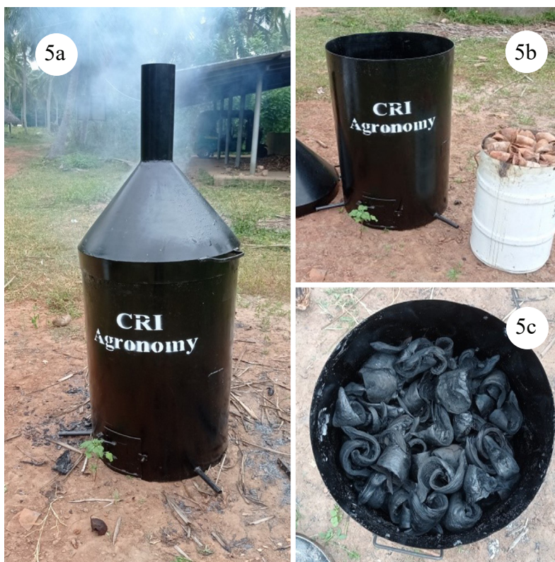
Fig 05. Biochar production at Rathmalagara Research Center (a) Mini Pyrolizer, (b) 1/4th cut size of king coconut husk as the feedstock and (c) Produced biochar from king coconut husk.
