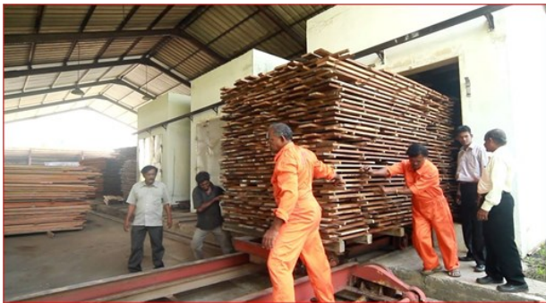
Preserving, curing and drying sawn timber.
