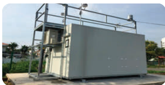
Permanent Air Quality Measuring Unit
