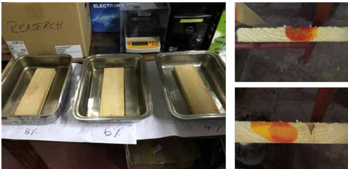
Conducting research on the effectiveness of different dipping concentrations of Boron for pine wood
