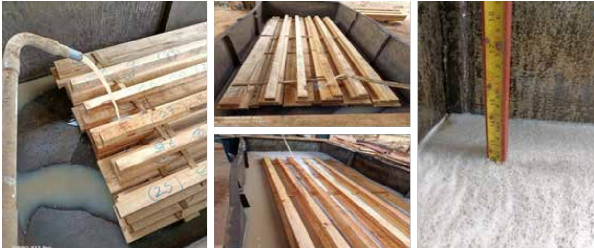
Conducting research on the effectiveness of different dipping periods of Boron for pine wood
