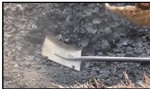
Figure 2.6 Coconut shell charcoal produced using the traditional method, Bopitiya Coconut Model Garden.
