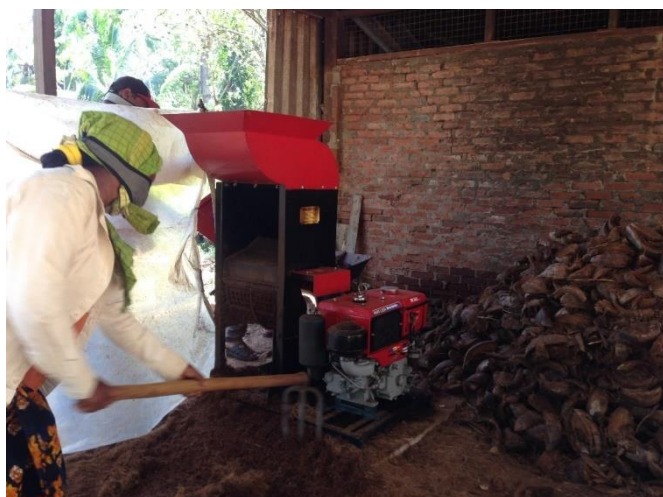
Figure 2.41 Chopping of husks by using the multi-chopper machine at Embilipitiya Nursery
