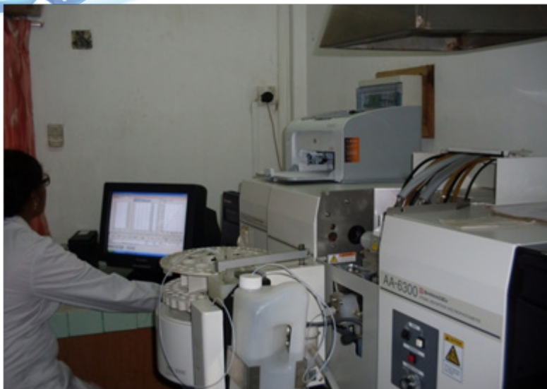
Fig 2: Instrument (Atomic Absorption Spectrophotometer) using for Heavy metal analysis in water samples.
