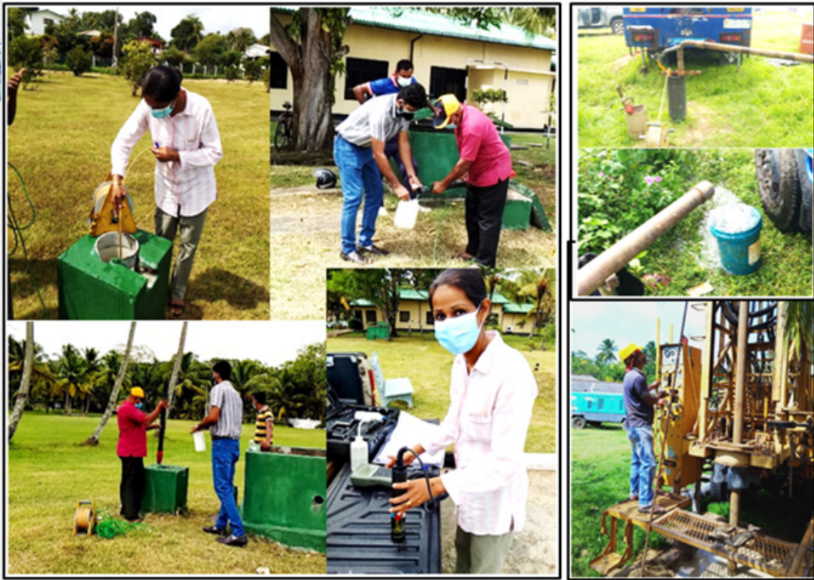
Figure 03: Project activities -measuring groundwater table, collecting of water samples, in-situ water sample analysis, test well drilling and aquifer testing
