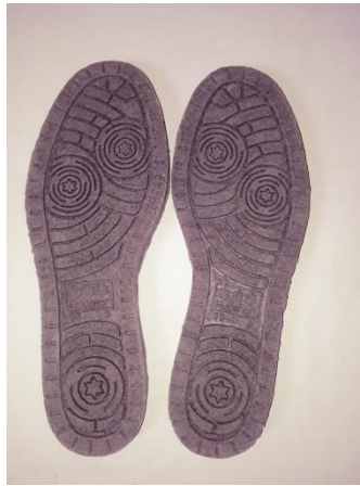
Fig. 2. NR based shoe soles produced with Durian husk fibres
