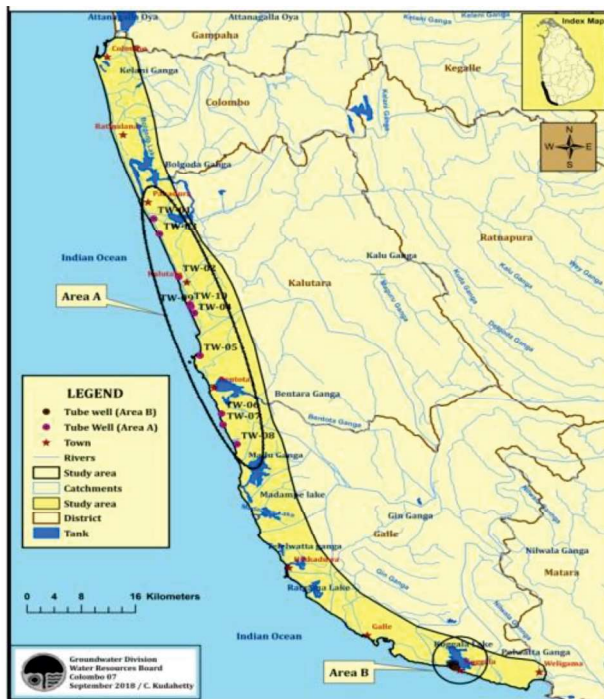
Figure 03 - 1: Established groundwater monitoring network areas, sampling and water level monitoring points. (Colombo to Weligama coastal strip)
