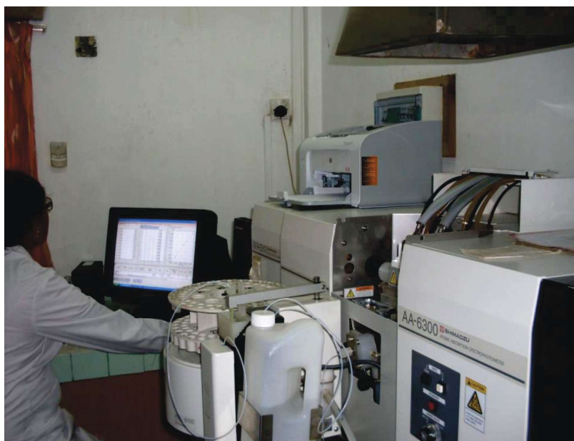
Fig 3: Instrument (Atomic Absorption Spectrophotometer) using for Heavy metal analysis in water samples.
