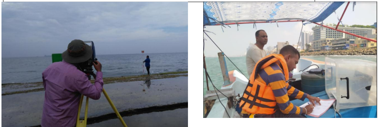
Figure 5:6 Land and bathymetric survey field work at Port City Development Project
