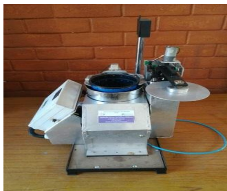
Instrument for measuring of Surface water level of tea leaves
