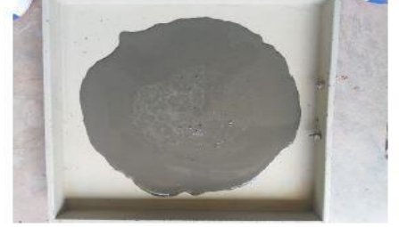
c) Water / Cement: 0.7 + 1% coir
