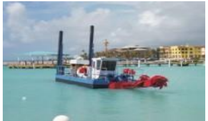
Nil Diyawara Cutter Suction Dredger
