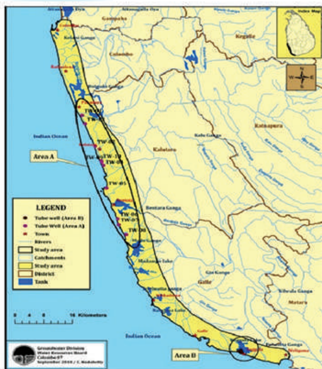
Figure 34: Established groundwater monitoring network (Colombo to Weligama coastal belt).
