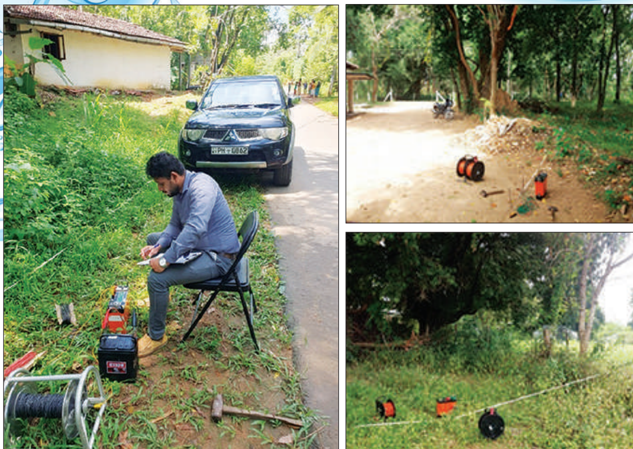
Figure 44: Conducting 1D resistivity survey to select suitable locations for tube well constructions
