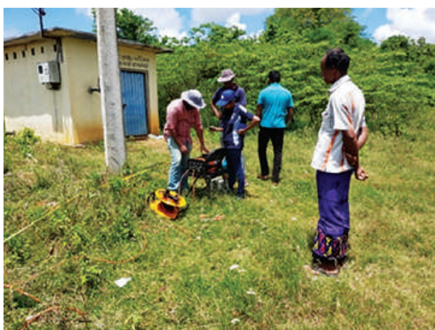
Figure 45: Conducting 2D geophysics and Field investigation tube well constructions
