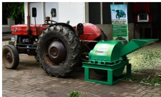
Shredder/Crusher Four-wheel tractor mounted (Large Scale)
