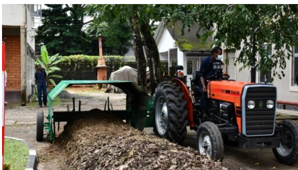
Compost Turner- Four-wheel tractor mounted (Large Scale)
