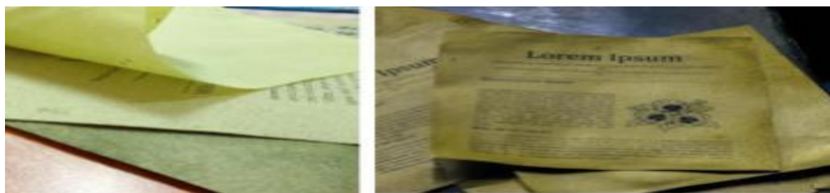
Figure 3-1 Eco-friendly packaging material made with fibres extracted from Water Hyacinth.
