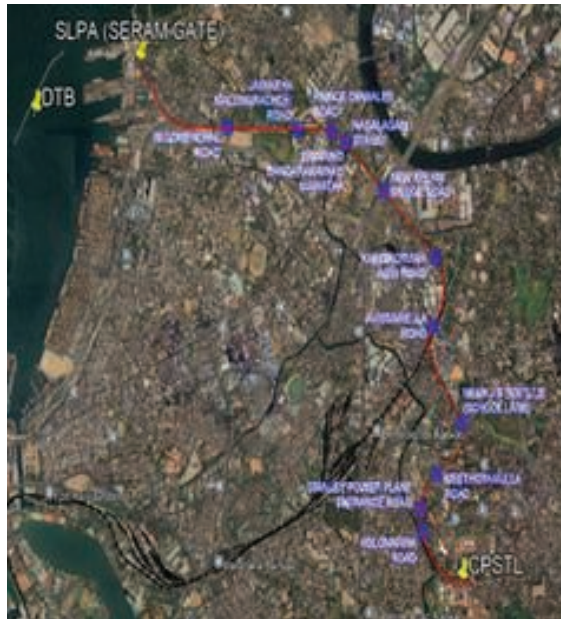
Proposed pipeline route from Kolonnawa Installation to SLPA Premises
