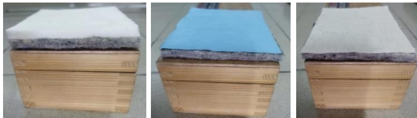
Composite materials produced with the NR latex based glue
