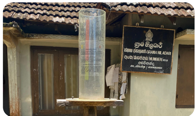
Manual Rain Gauges Installed under CBDRM Program
