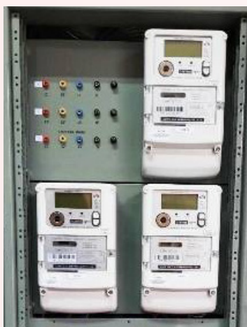
Front panel of the distribution line model designed to test voltage violations and mitigation methods
