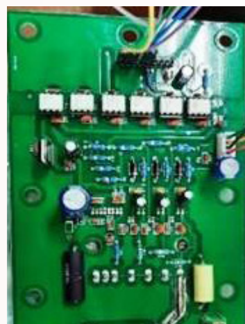
Fabricated circuit for re-phasing inverter
