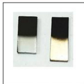
Counter electrodes for dye solar cells, prepared using activated carbon and sugar composite on conducting glass substrate and
