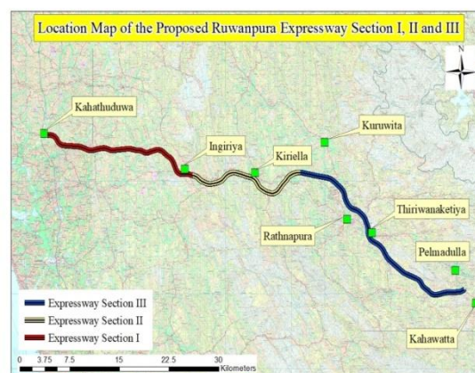
Figure 01: Proposed Trace for Ruwanpura Expressway Project
