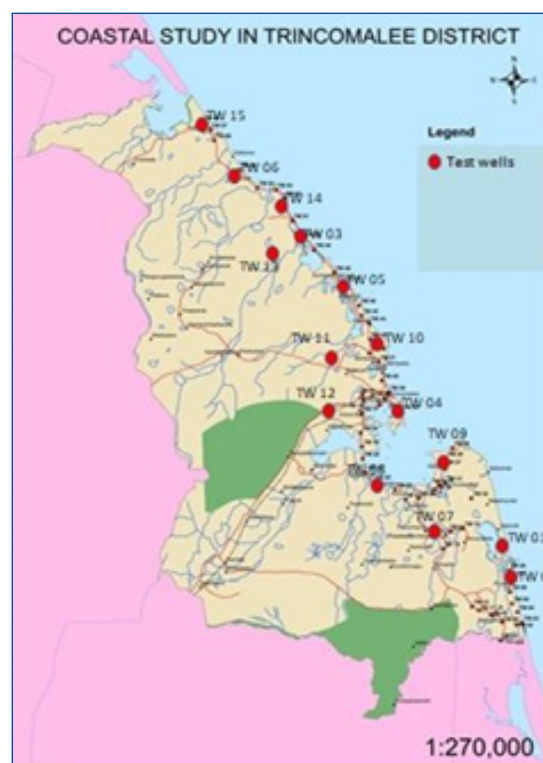
Figure 18: Established groundwater monitoring network (Trincomalee coastal belt).
