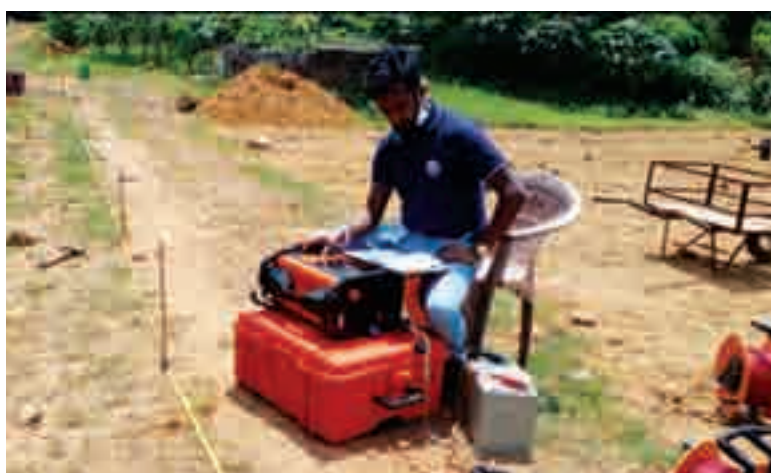
Figure 39: Conducting 1D resistivity surveys to understand about the sub surface conditions.
