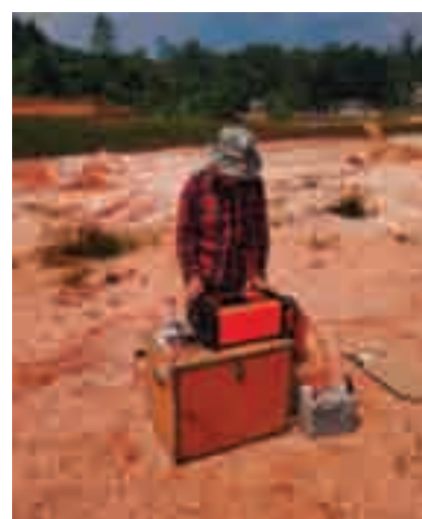
Figure 40: Conducting 2D resistivity surveys in central highway trace to understand about the sub surface
