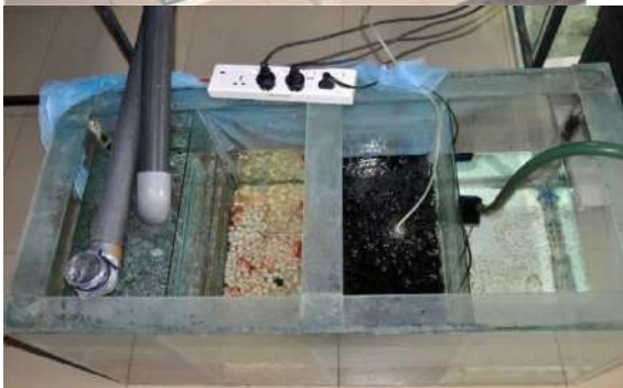
Figure 7: Newly designed filter unit of RAS system
