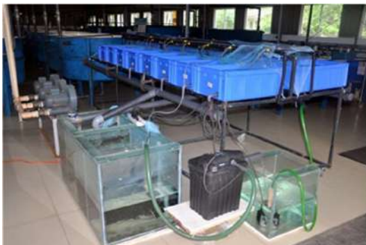
Figure 6: Newly designed RAS system
