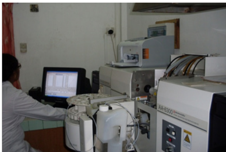
Fig 2: Instrument (Atomic Absorption Spectrophotometer) using for Heavy metal analysis in water samples.
