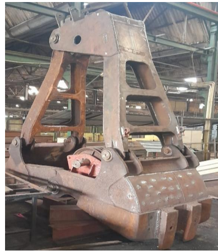
Grab Bucket Repair
