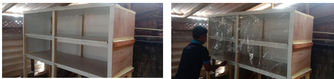
Figure 3: Wooden rack designed for growing algae
