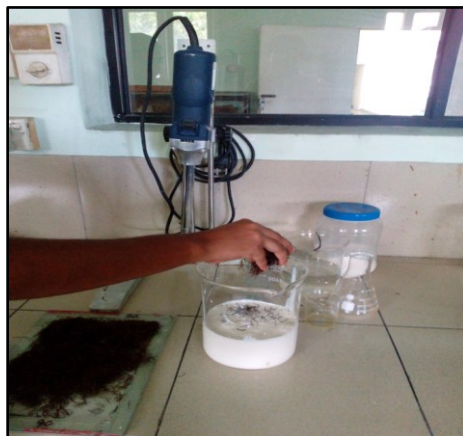
Surface treatment of palmyra fibres with latex to produce palmyra fibre-natural rubber (NR)-styrene-butadiene rubber (SBR) composites
