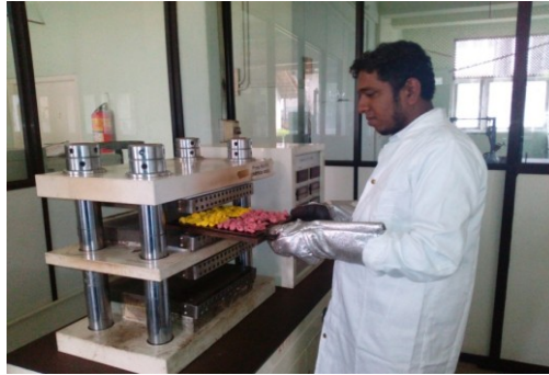
Compression moulding of natural rubber (NR)-low density polyethylene (LDPE) composites using a press machine
