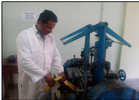
Preparation of the low resilient and high abrasion resistant rubber ball compound using a two-roll mill
