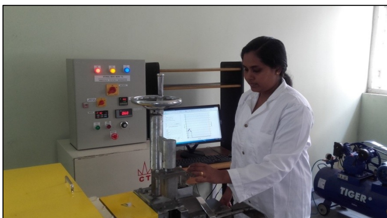
Preparation of rubber and rubber-plastic composites using the newly purchased computerized laboratory scale internal mixer
