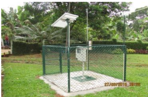
Installation of automated rain gauges in progress in Elpitiya and Ingiriya
